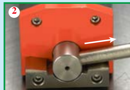
Pull out the lever Tire le levier
