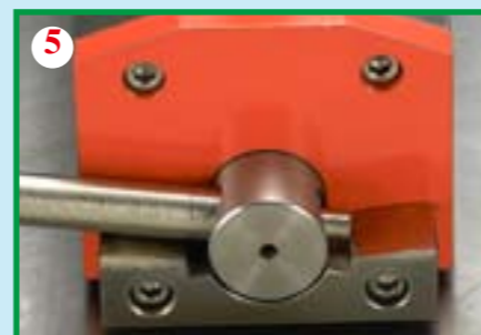
Lever locked in "ON" position Levier verrouillé en position "ON"
